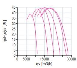
measured in full bell mouth without guard grille in installation type A according to ISO 5801 Please note: It's not allowed to use this fan in the stall area!\*
