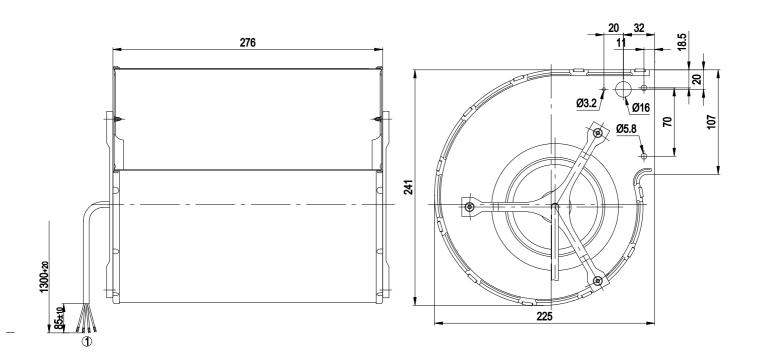
Connection line ETFE AWG 20, 4x brass lead tips crimped
